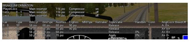
All of the hoses are now connected; only the angle cocks on the lead locomotive and the last car are closed as indicated by the –. The rest of the cocks are open (+) and the air hoses are joined together (all I) to connect to the air supply on the lead locomotive.
