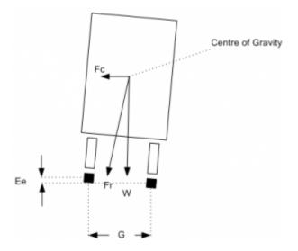
Fig. 3: Forces on rolling stock transitioning a curve
