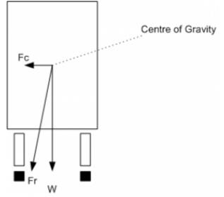
Fig. 5: Forces at work when a train rounds a curve
