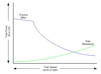
The first force is the tractive effort produced by the locomotive, whilst the second force is the resistance presented by the train. Whenever the tractive effort is greater than the train resistance the train will continue to move forward; once the resistance exceeds the tractive effort, then the train will start to slow down, and eventually will stop moving forward.
